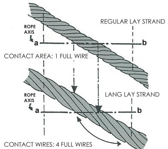
The above is a comparison of wear characteristics between regular lay and lang lay ropes. The greater metal area along the rope's axis (a-b) promotes more wear-resistance than a regular lay rope. The longer exposed length of outer wires in a lang lay rope offers an easier bend, resulting in greater fatigue resistance (page 9).
