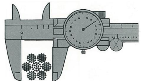
The true diameter of wire rope is measured at it's largest point.
