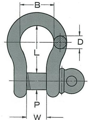
Above working load limit is based on a design factor of 6:1.
