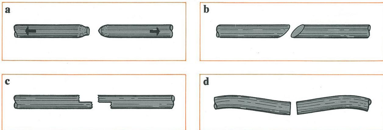
A wire broken under a tensile load that exceeds its strength is recognized by the “cup and cone” configuration at the fracture point (a). The *necking down* of the wire at this point shows that failure occurred while the wire retained its ductility. Shear-tensile fracture (b) occurs in wire subjected to a combination of transverse and axial loads. Fatigue breaks are usually characterized by squared-off ends perpendicular to the wire either straight across or Z-shaped (c & d).
