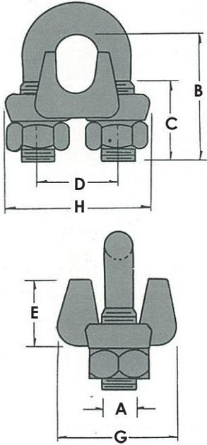
**Drop-Forged Wire Rope Clips**
