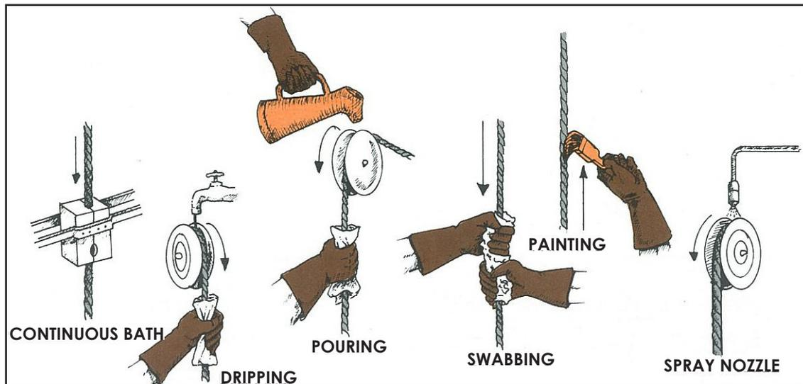
The illustrations above are proper methods of applying lubrication to a rope in service. The arrows indicate the direction of the ropes' movement.
