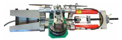
Image shows the Petersen P400 Swaging System, allowing proof load testing to be completed at time of swaging.
